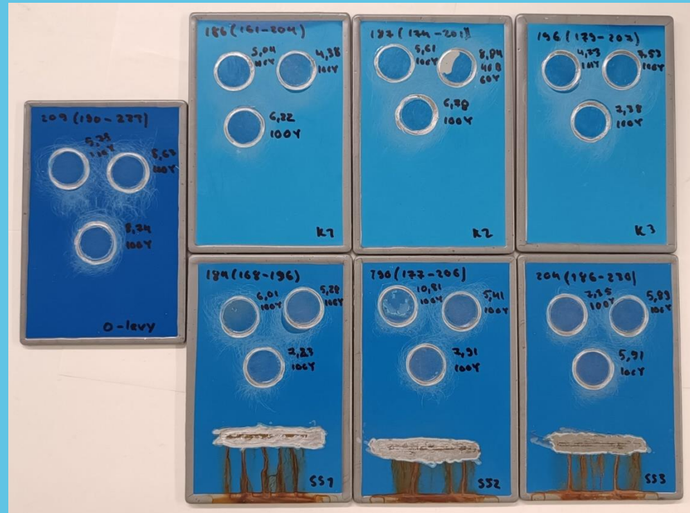
C5M: Epocoat Aqua Pr 80 µm + Norepox Aqua DTM 100 µm
